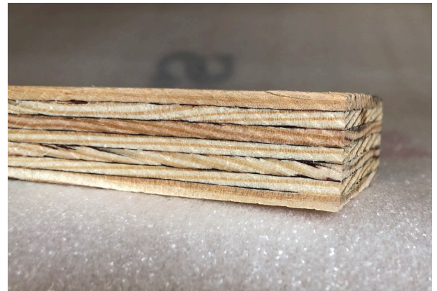
Plywood; made from layers of the same thickness using similar types of wood to produce a stable material.
