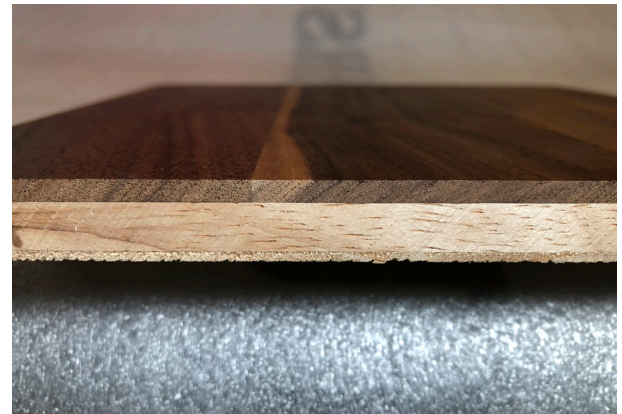
Typical Engineered floorboard; different types of timber with different movement characteristics in layers of different thicknesses. Board cannot be considered stable compared with plywood.
